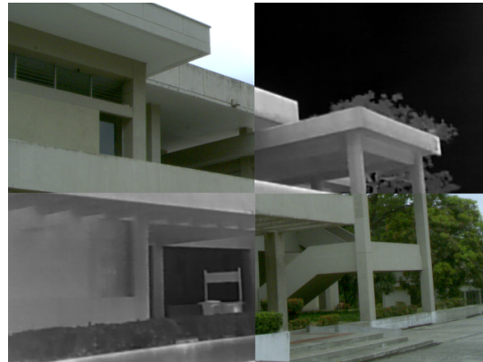
Figure 1. A montage of visible and thermal images, captured from the same point of view but with different cameras sensor [35].
