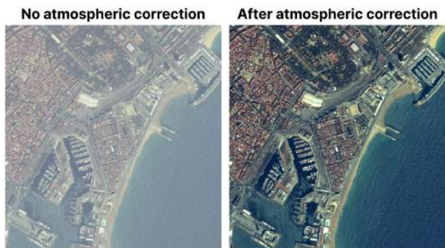
Fig. 14. Comparative example of the effect of atmospheric correction on a satellite image.
