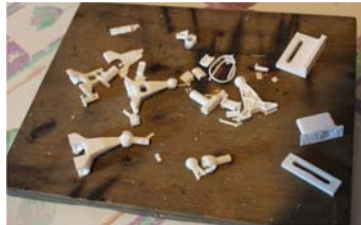
Fig. 6. ABS/PLA 3D printed parts as elements for the material characterization
