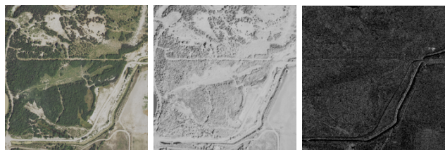
Figure 4. Example stack (RGB, IR, SAR), made from aligning UMBRA and HRO data.
