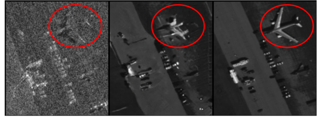
Figure 3. Example of failed translation from SAR to EO (order = SAR input, translation, ground truth). We draw attention to the aircraft in the image. The translated image illustrates an example of the generative network hallucinating.
