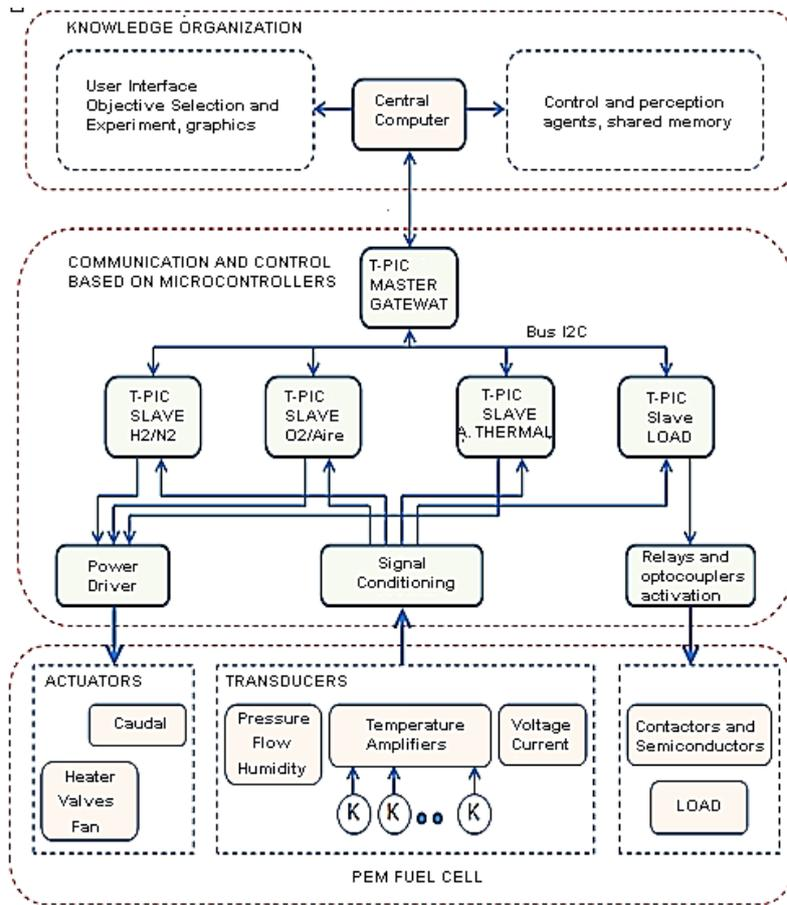
Fig. 6. Distributed network of nodes for monitoring and control of the PEM stack.
