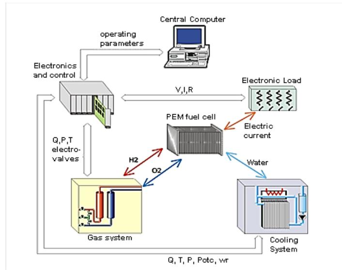
Fig. 1. Structure of integration subsystems that make up the system for the integrated control of the PEM stack.
