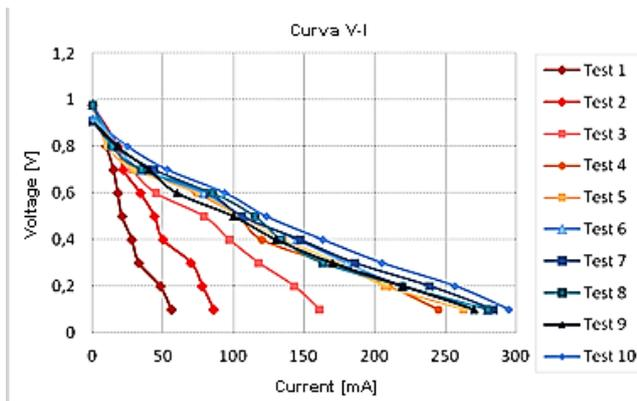
Fig. 9. Polarization curves obtained from a PEM fuel cell.
