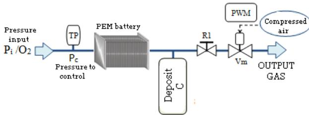
Fig. 2. Pressure regulation system by PWM online.
