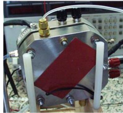
Fig. 3. Heating mat used to raise the temperature of the PEM stack of low power.
