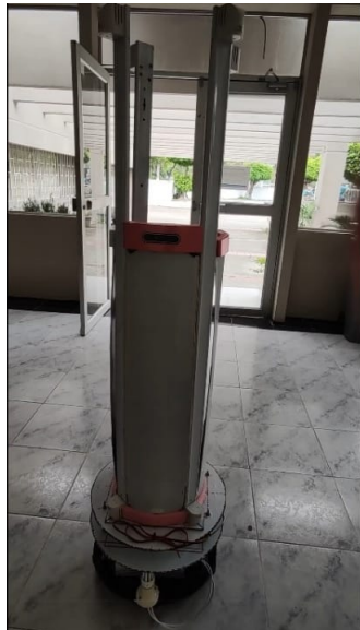
Fig. 2. UVC System implemented in a differential robot
