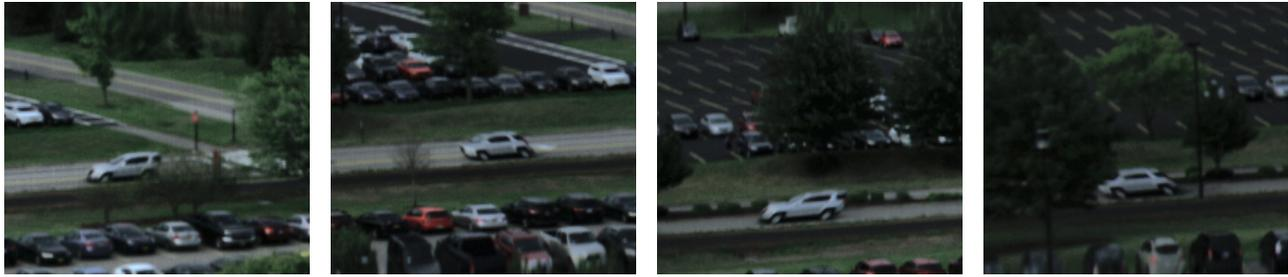
(a) Set of ordered frames from the dataset: the vehicle, along with others in the dataset, appears distorted once the push-broom tilt sweep is complete and all lines stitched together depending on their relative speed to the camera’s frame rate and its tilt motion.
