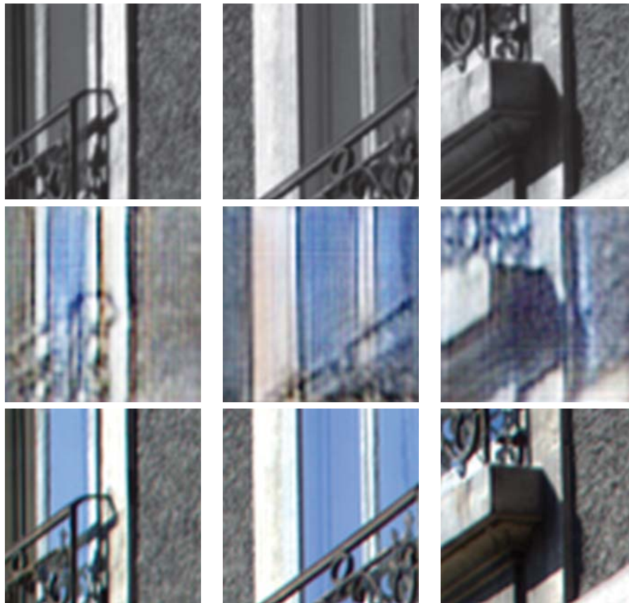
Figure 4.11 – Results obtained with the second approach: ( top ) NIR images from the urban category; ( middle ) Images colorized with the DCGAN network trained with urban Images; ( bottom ) Ground truth images.
