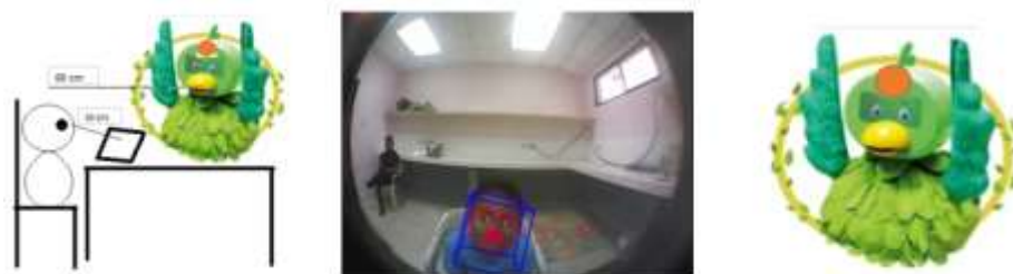
Fig. 3. Interaction scenario: a) General scheme; b) Frame captured by LOLY's camera; and c) Camera location in LOLY
