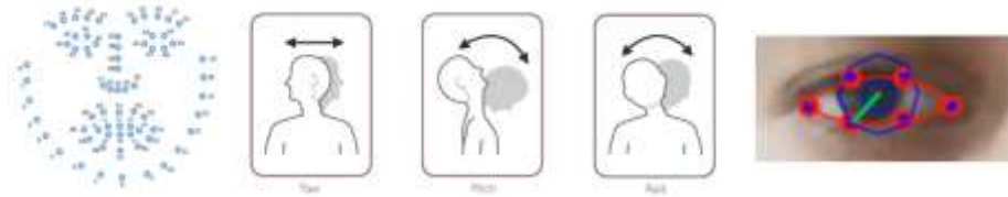
Fig. 2. Facial Points / Head Movement / Eye Gaze - OpenFace
