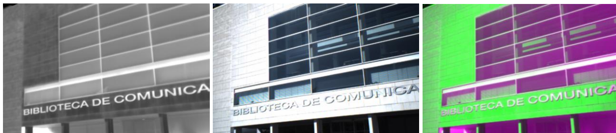
Fig. 3. (left) Input LWIR image. (middle) Input VS image. (right) Result from the MI Registration (input images are overlapped using different colours to appreciate the results).
