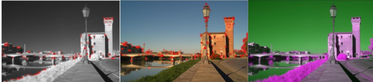
Fig. 2. Registration of NIR and VS images. (left) NIR image with selected keypoints; (middle) VS image with selected keypoints; (right) Registration result obtained by minimizing MSE over selected keypoints ( this figure is best viewed in color ).
