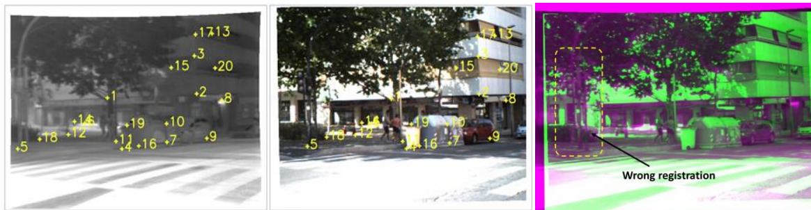
Fig. 1. Registration of LWIR and VS images. (left) LWIR image with the set of keypoints (20 points); (middle) VS image with the corresponding keypoints (20 points); (right) Registration result obtained by minimizing MSE ( this figure is best viewed in color ).
