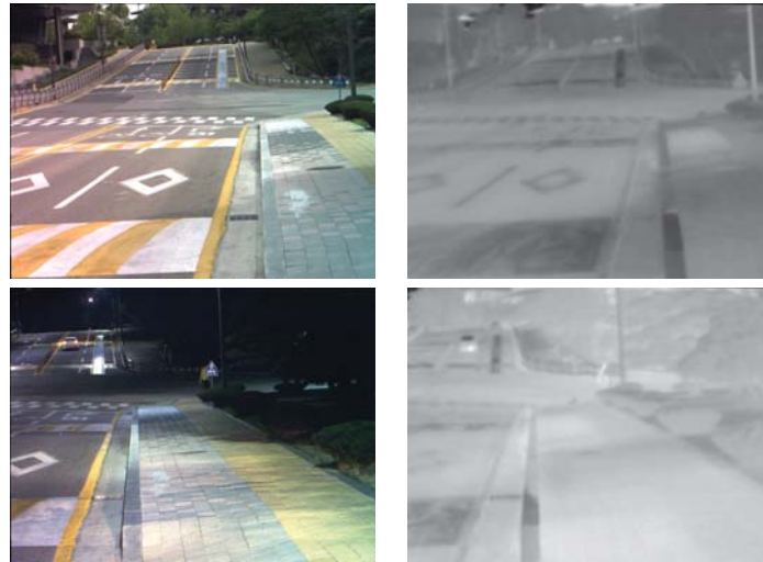
Figure 8. Three pairs of cross-spectral images of the same scene but at different day-time (images from [8]): (Left) VS; (Right) LWIR.
